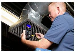
Type K Thermocouple Input for differential temperature measurements
